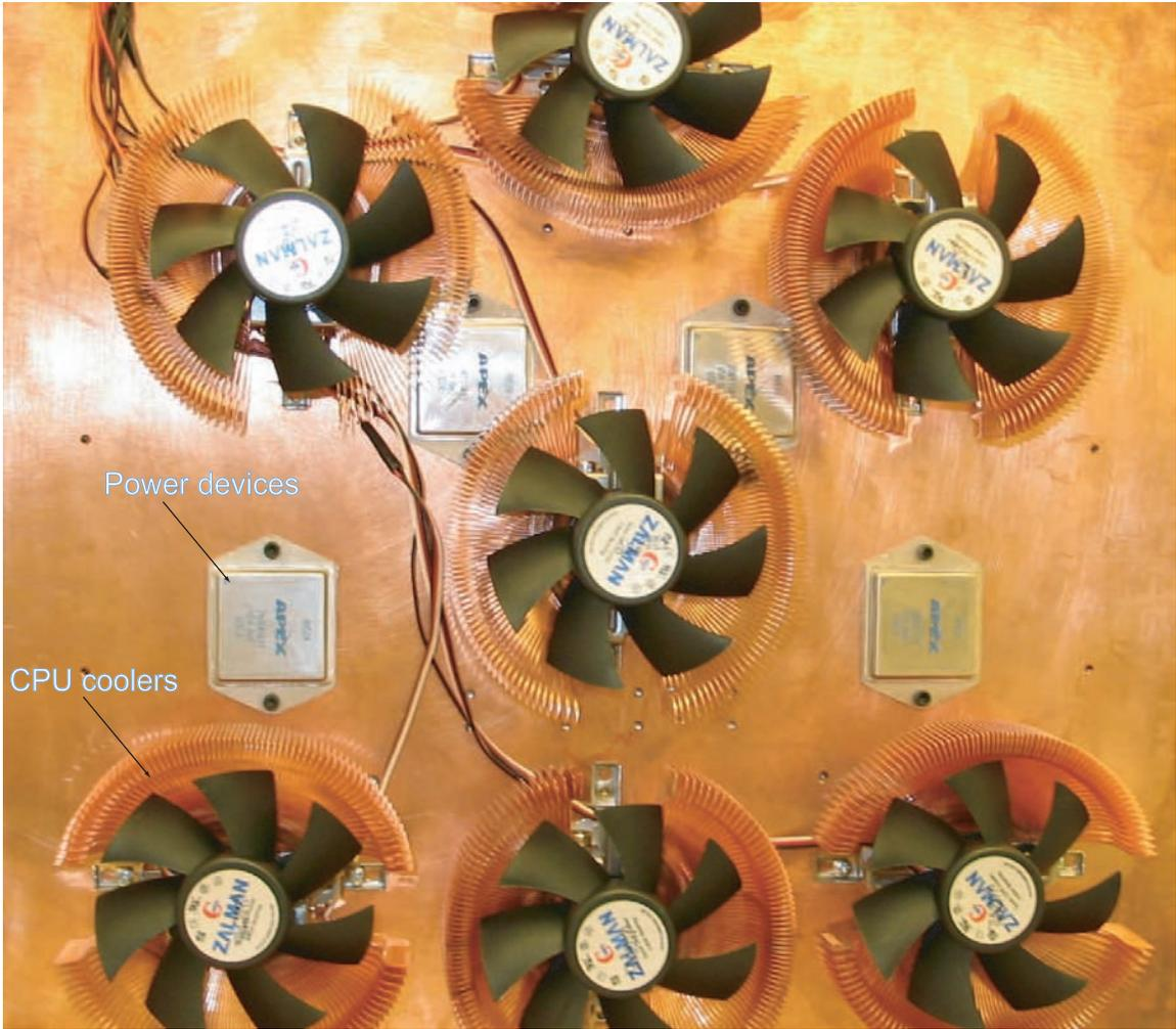
Figure 5-5: The heat sink of the power amplifier
