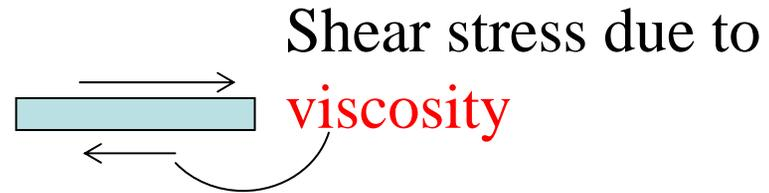
Shear stress  $\sim$  vel gradient  $\times$  viscosity
