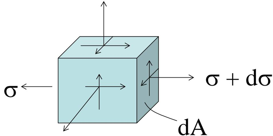
$$(\sigma + d\sigma - \sigma)dA + \text{force from other faces} = \text{mass} \times \text{accel} + \text{body forces} \quad (\text{e.g wt.})$$
