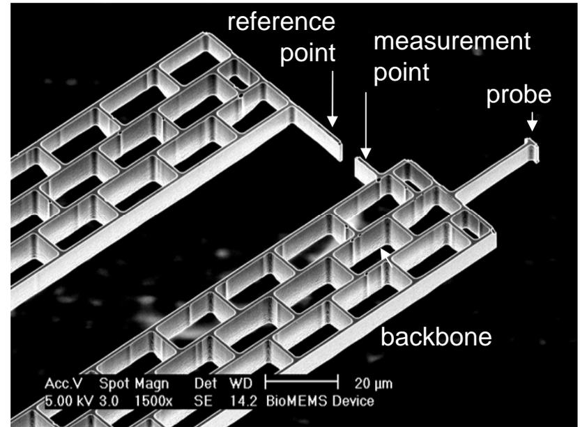
**sensor beams: 2 mm x 1  $\mu$ m x 10  $\mu$ m,**
