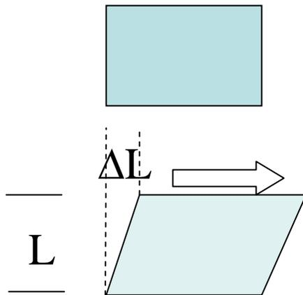
**Shear strain =  $\Delta L/L$**
