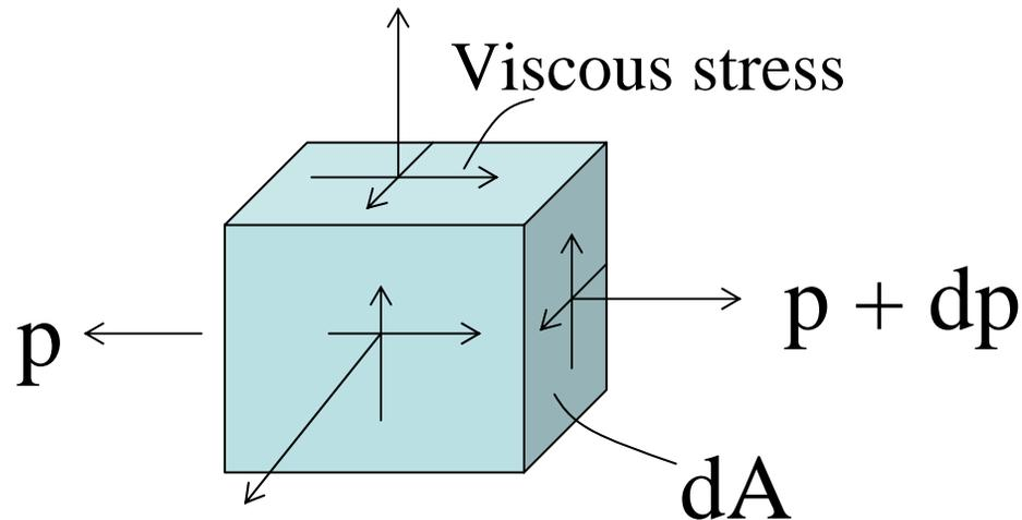
Viscous force + pressure force + body force = mass  $\times$  accl.
