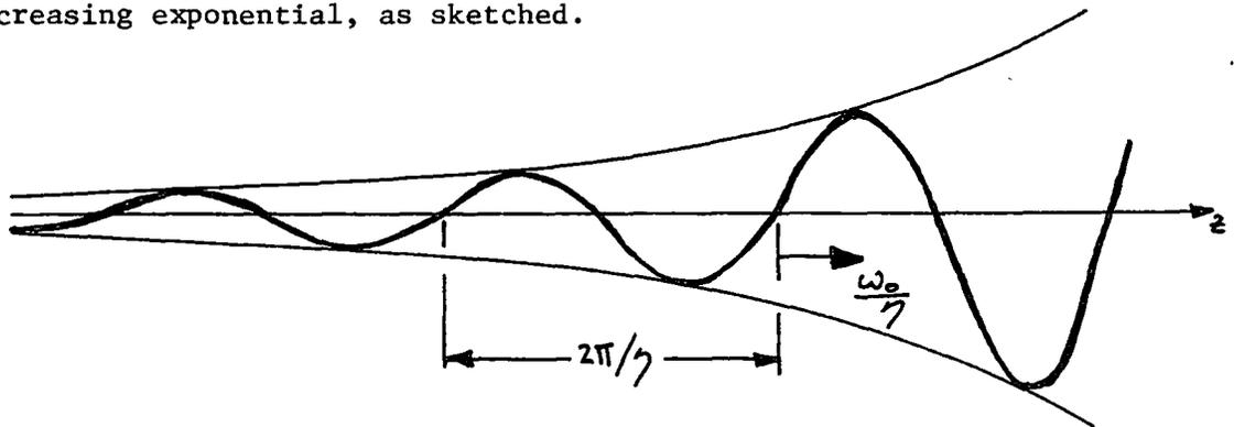
This is illustrated by the experiment of Fig. 11.11.5. If the frequency is so high that  $\omega_0^2 + P(1-M^2) > 0$ , the envelope is a standing wave
