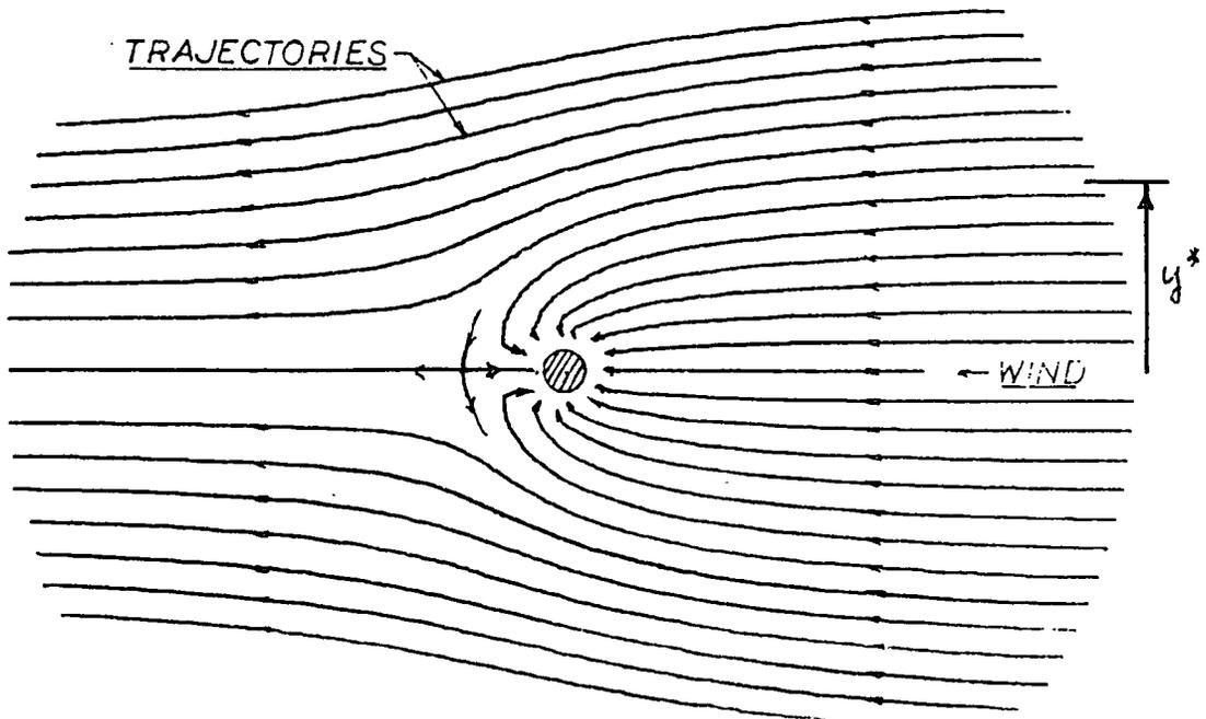
Negative Particle Trajectories for a Positive Conductor in the Stationary Flow Case (Attracted Particles)
