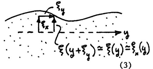
Prob. 8.16.4 (cont.) Boundary conditions on the fields in the gas recognize that the electrode and the interface are each equipotentials.
