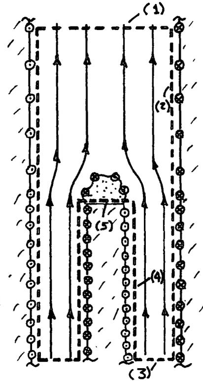
Prob. 3.10.4 The electric field is sketched in the figure. The force on the cap should be upward. To find this force use the surface  $S$  shown to enclose the cap. On  $S_1$  the field is zero. On  $S_2$  and  $S_3$  the electric shear stress is zero because it is an equipotential and hence can support no tangential  $\vec{E}$ . On  $S_4$  the field is zero. Finally, on  $S_5$  the field is that of infinite coaxial conductors.
