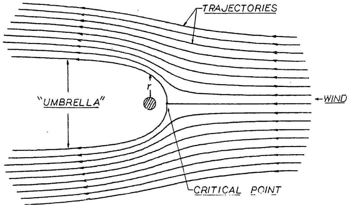
Positive Particle Trajectories for a Positive Conductor in the Stationary Flow Case (Repelled Particles)
