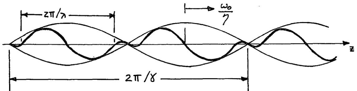
Note that at cut-off, where  $\omega_0^2 = P(M^2 - 1)$ , the envelope has an infinite wavelength. As the frequency is raised, this wavelength shortens. This is illustrated with  $P = 0$  by the experiment of Fig. 11.11.4.
