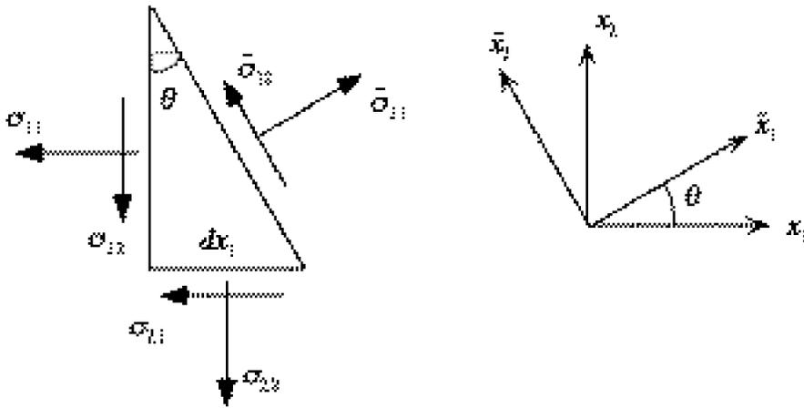
Find the values of  $\theta$  that produce the maximum and minimum values of  $\bar{\sigma}_{11}$ , what are the corresponding values of  $\bar{\sigma}_{12}$ ? Do not try to distinguish between the maximum and minimum values.
