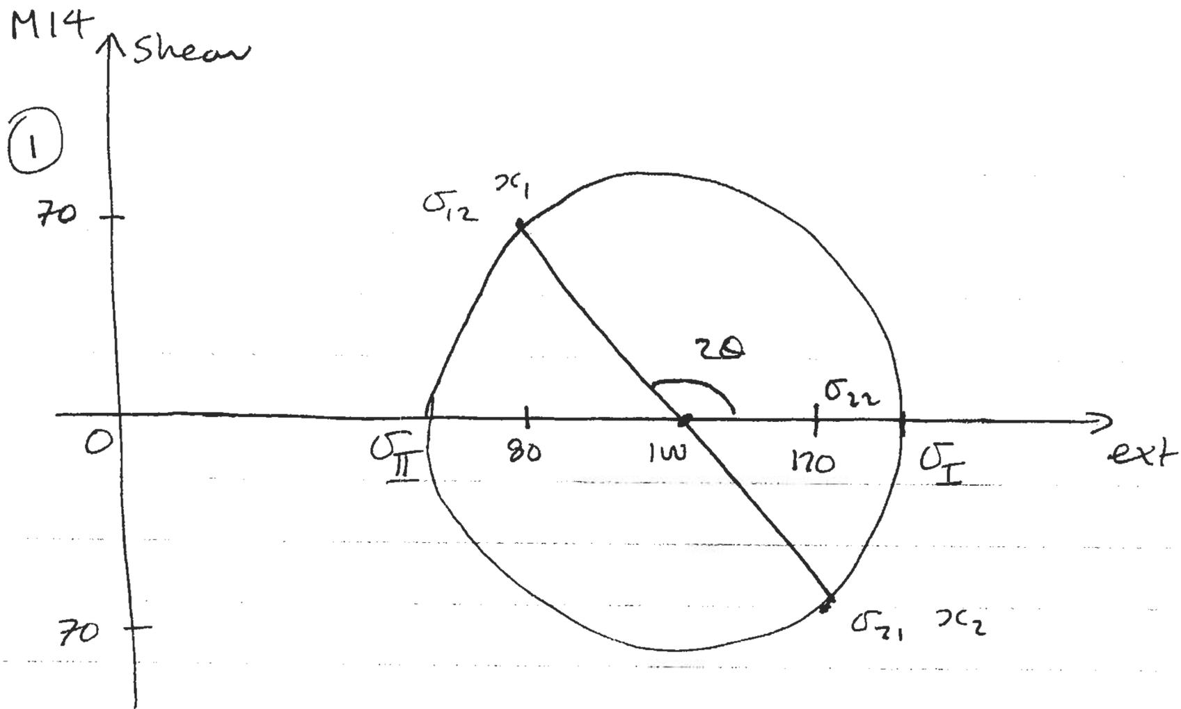
$$\text{Radius} = \sqrt{20^2 + 70^2} = 72.8 \text{ MPa} = \text{Max Shear}$$
