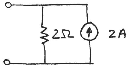
2. As above, apply a test current. This time, I'll use node method. (There are more unknown nodes with node method, but the loop method is trickier, due to current source in circuit.)
