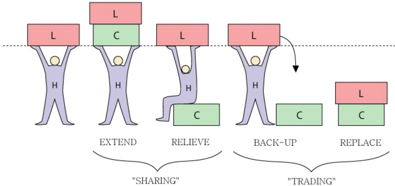
The notions of trading and sharing control between human and computer. *L* is the load or task, *H* the human, *C* the computer. [Adapted from W.Verplank.]
