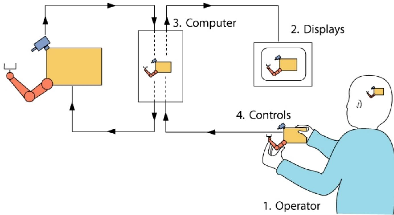
Four loci of models in the supervisory control system: (1) Mental Model (2) Display Representation (3) Control Configuration (4) Computer Model. (Adapted from W. Verplank.)
