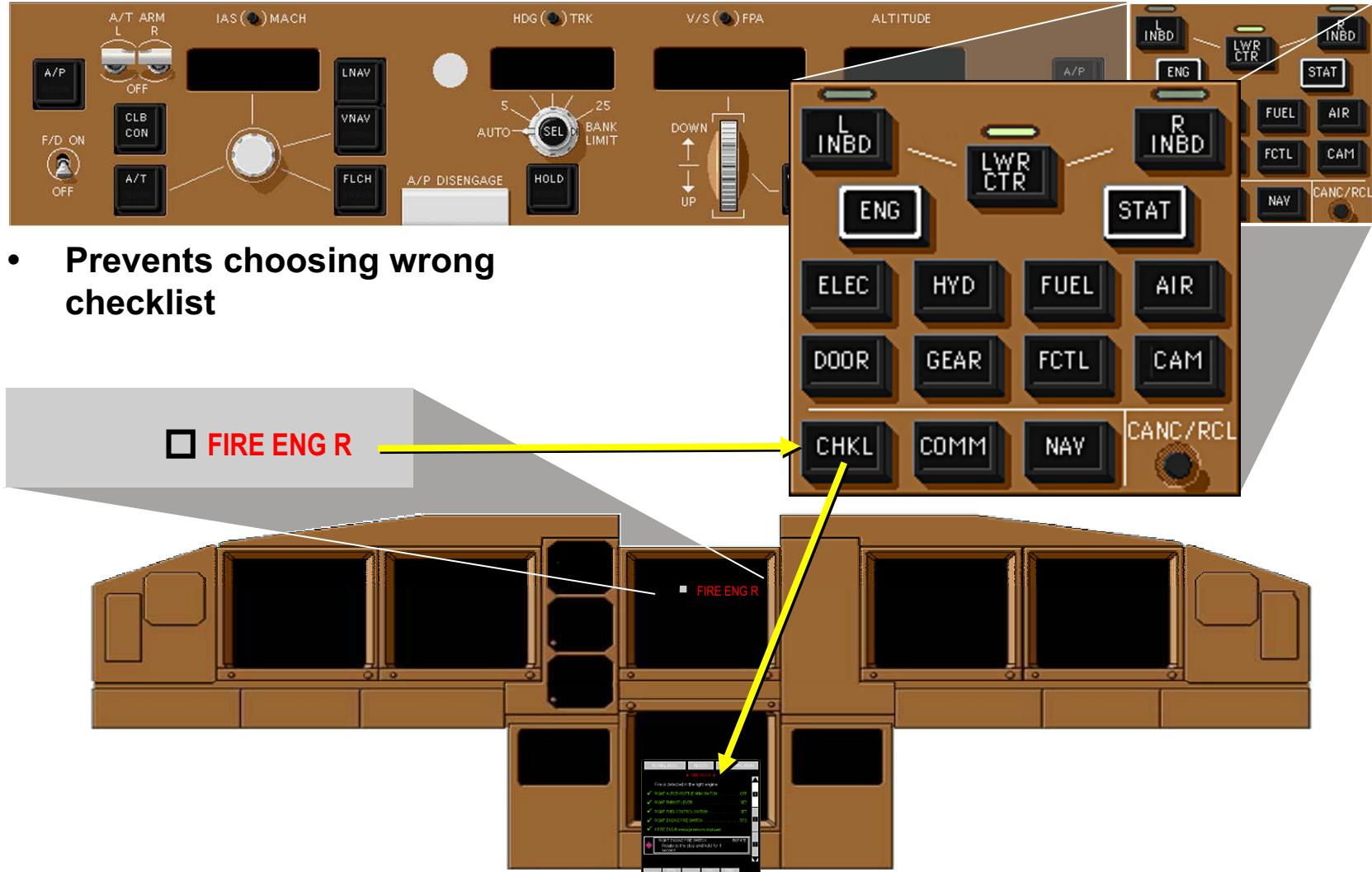
When an alert message is displayed, the pilot simply pushes the CHKL button and the correct non-normal checklist is displayed. This prevents the crew from accidentally choosing the wrong checklist.
