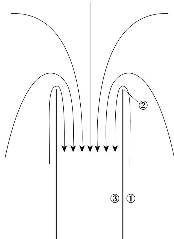
For high Re, BL thin  $\implies$  streamlines for flow into pipe will follow geometry
