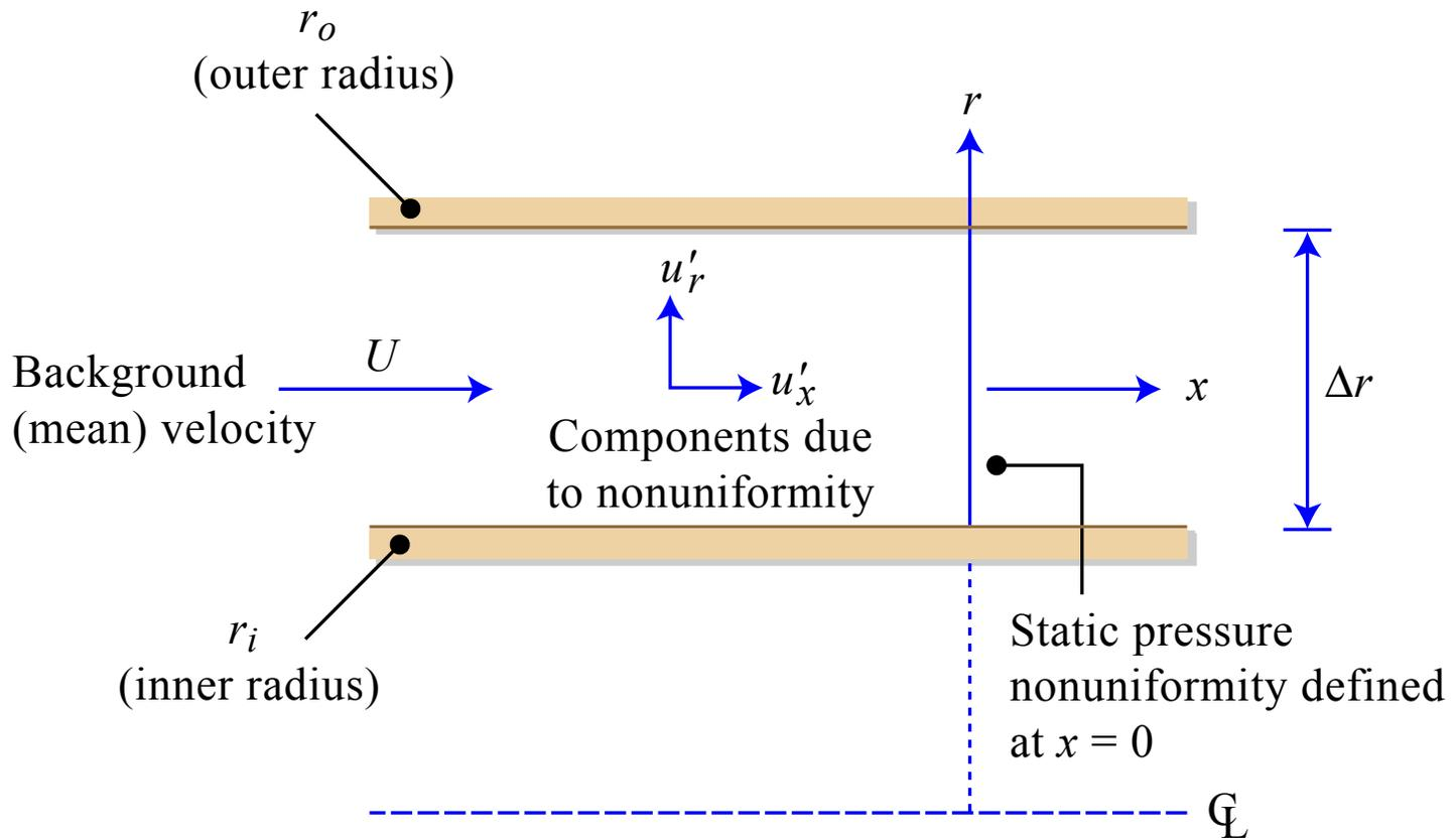
Annular flow geometry used in estimation of upstream influence region for axisymmetric flow; region of interest is  $x < 0$ .
