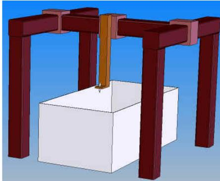
Floor-mounted gantry with separate cutting table
