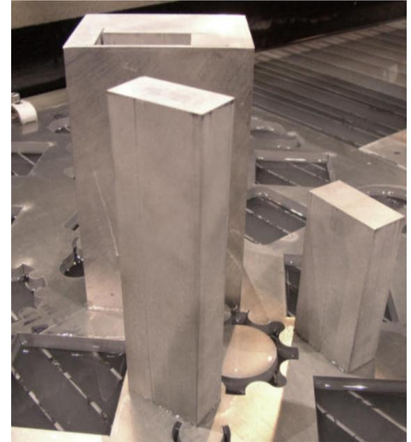
*This piece was made from 8" (200mm) thick aluminum as a demonstration of what an abrasivejet can do*
