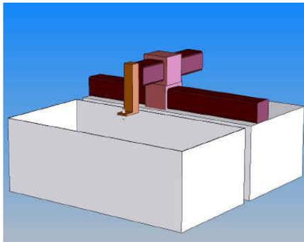
Floor-mounted cantilever system with separate cutting table
