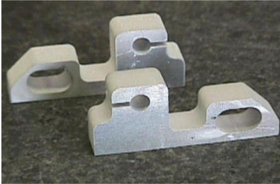
*An example of two aluminum parts done in 1/2" (1.3 cm) thick aluminum, which took approximately five minutes to machine*
