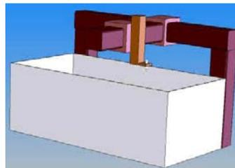
**Dis:** Y-axis is limited in length to about 5 feet because of structural considerations
