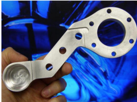
*A prototype linkage arm for the Tilt-A-Jet. This part was first "roughed out" on the OMAX. The holes were then reamed out to tolerance, and some additional features (such as pockets) added with other machining processes.*
