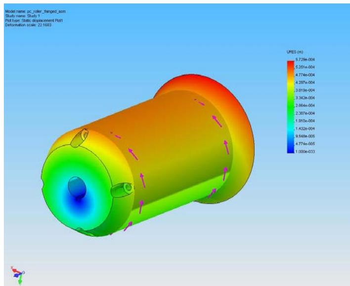
**Figure 12: Drive Roller Displacement**
