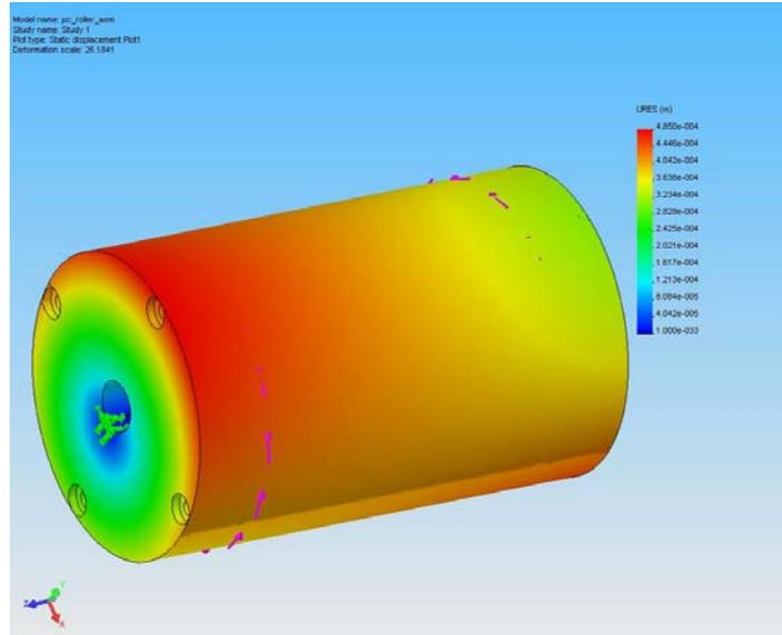
**Figure 9: Drive Roller Displacement**
