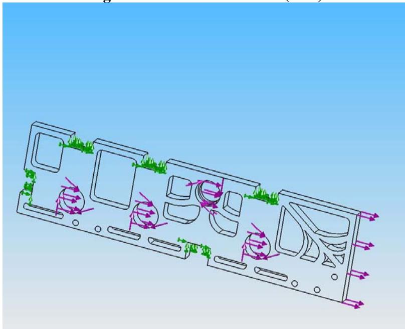
**Figure 14: Side Plate Forces (Right)**
