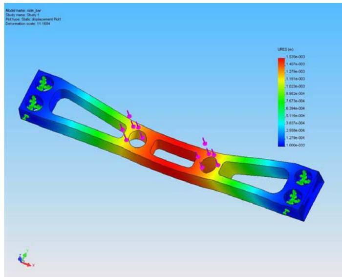
**Figure 6: Cross Side Bar Displacement**
