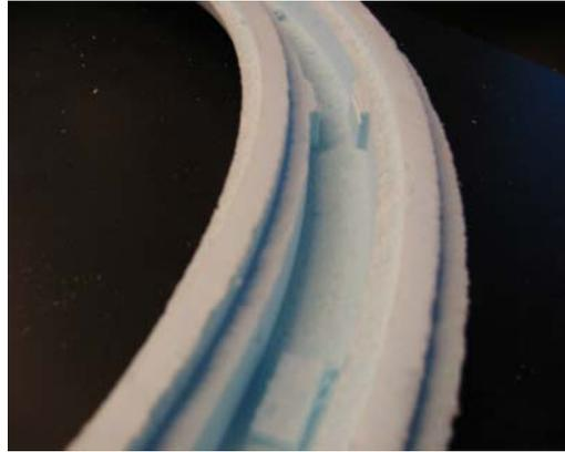
**Figure F.7-D: Spacers for the Male Part of the Container**
