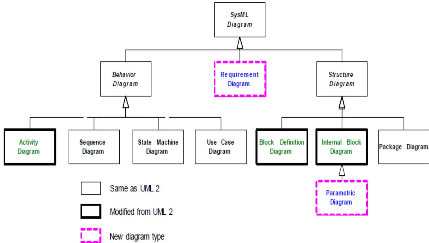
The types of SysML diagrams
