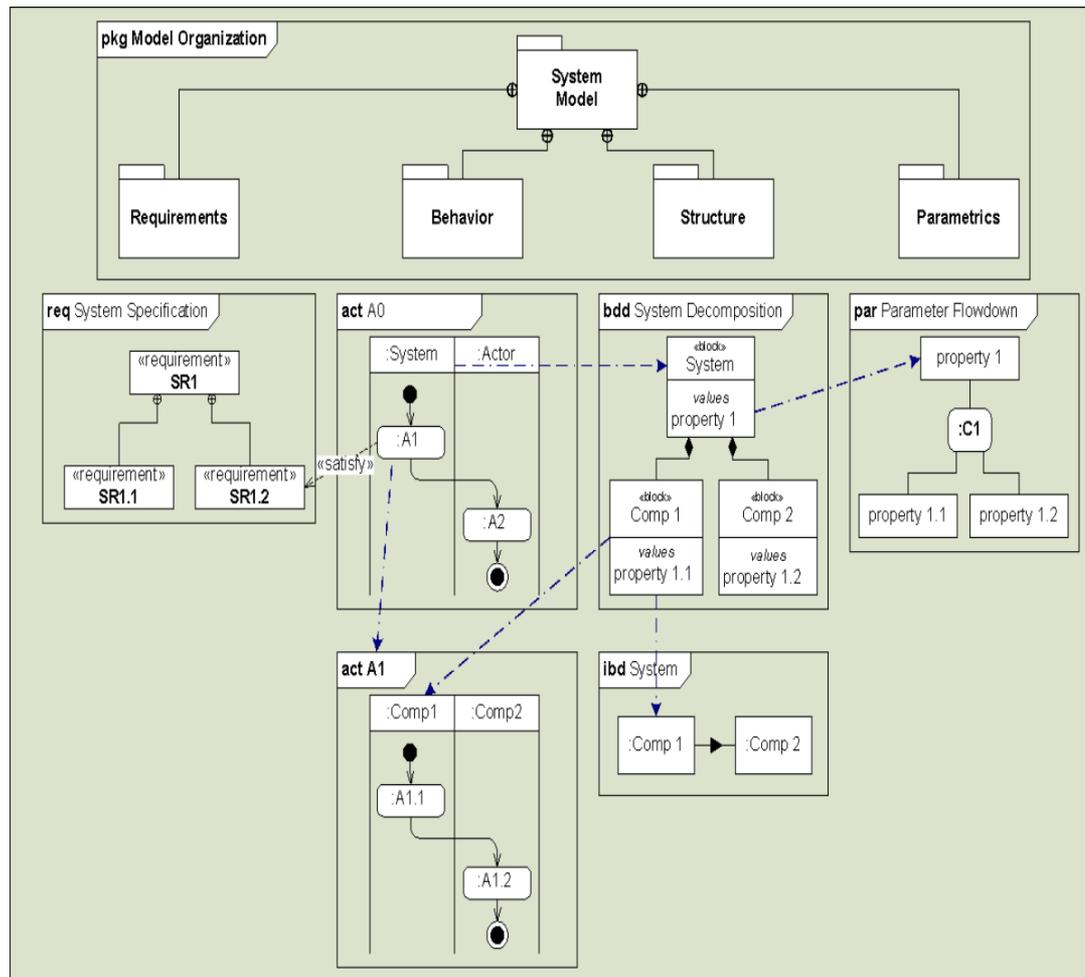
**SysML diagrams capture different types of system information. Diagrams can be linked together**
