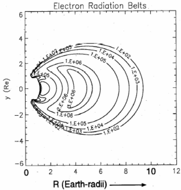
For the calculations required in this report, an estimate of the radiation flux for a given range of Earth radii are taken from Figures 1 and 2 by inspection. Figure 3 shows the worst-case radiation doses from both electrons and protons for a range of Earth radii. Although, Figure 3 does not span the entire range given in Figures 1 and 2, it yields a representative sample for the orbits considered in this memo.
