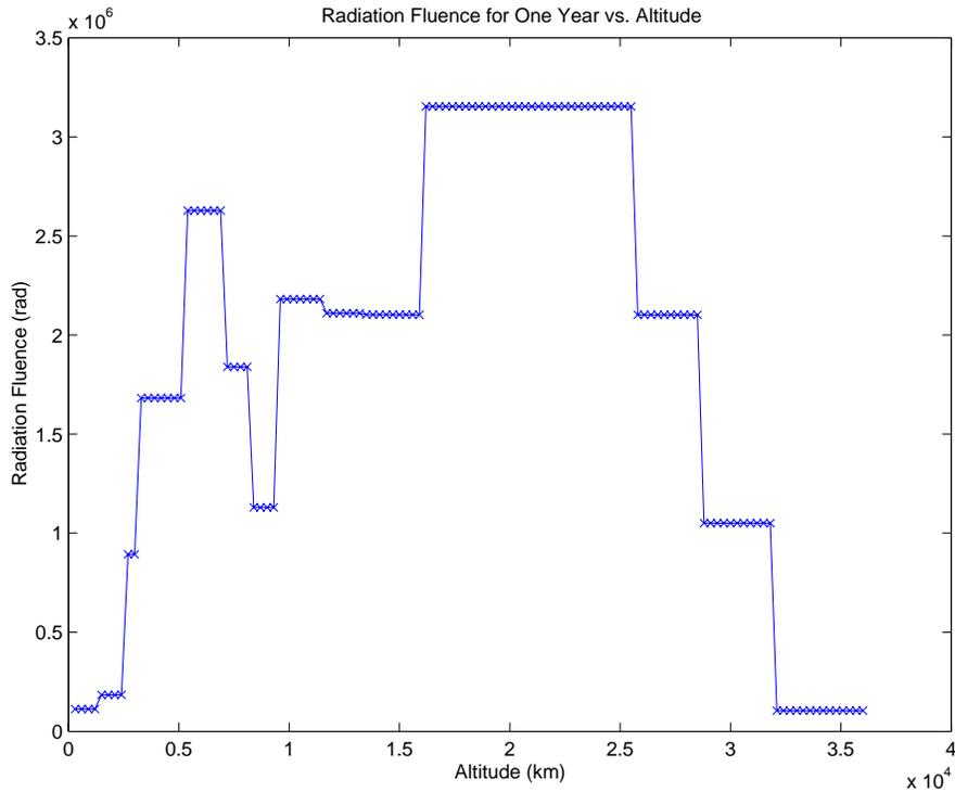
For the purposes of this research, a script was created that calculates the flux due to each particle and the total fluence accumulated in a specified time period (one year for this work). In this investigation, the primary interest is for three circular orbits; at LEO (300 km alt), at MEO (8000 km alt), and at GEO (36000 km alt). Table 2 gives the calculated flux and fluence over one year for each orbit considered.
