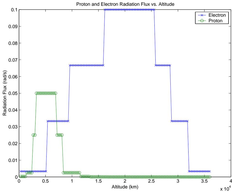
The radiation fluence is the integral of flux over time. For a circular orbit, the flux is considered constant, since the altitude is constant. Thus the radiation fluence is just the radiation flux time the time. Figure 4 gives the radiation fluence in a year for a range of altitudes.
