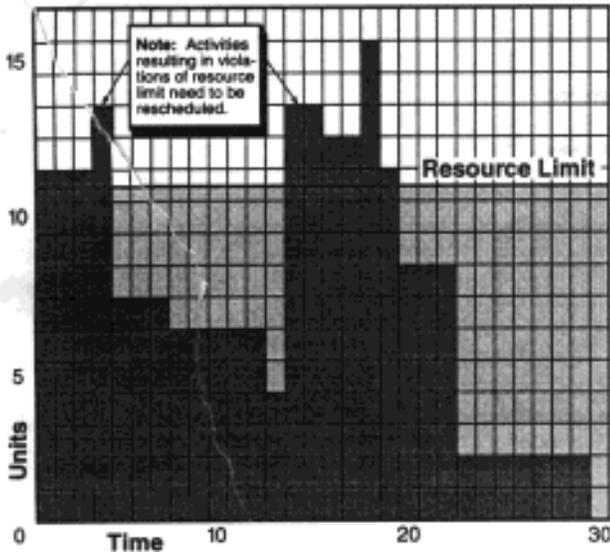
Figure 14 -- An Example of an Unlevelled Resource Profile.
