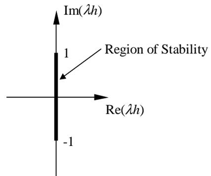
One may note that  $\lambda_j$  is always real and negative, thereby satisfying the criterion for stability of the space discretization of a parabolic PDE, keeping time continuous.
