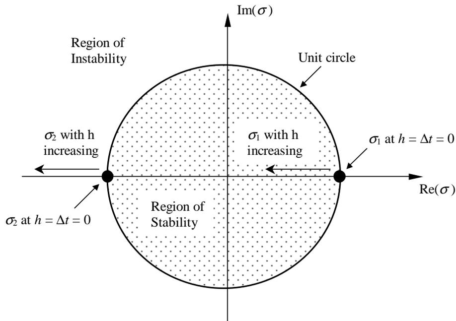
In this case,  $\sigma_1$  and  $\sigma_2$  start out being on the unit circle ( $h = \Delta t = 0$ ). However, the spurious root (refer to following slide) leaves the unit circle as  $h$  starts increasing. Therefore, the spurious root causes the leapfrog time discretization scheme to be unstable, irrespective of how small  $h = \Delta t$  is, although it does not affect the accuracy. The leapfrog time discretization for the 1-D Diffusion Equation is **unstable**.
