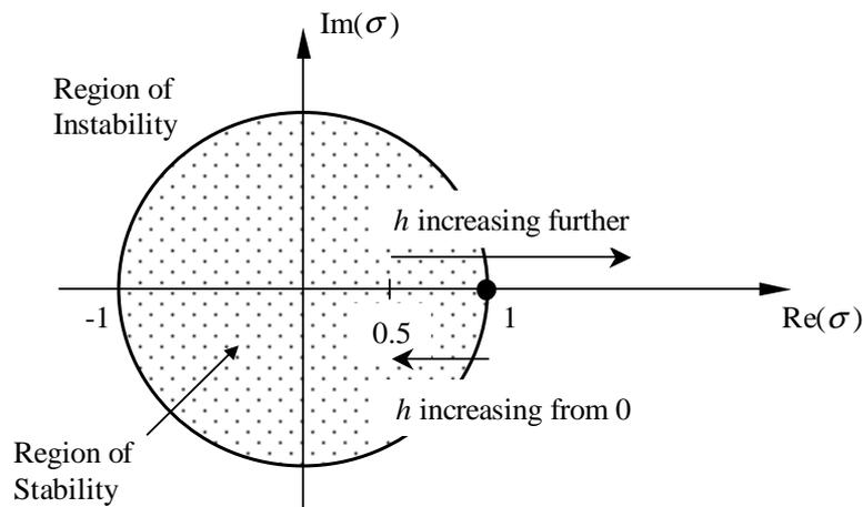
When  $h$  increases from zero,  $\sigma$  decreases from 1.0. As  $h$  continues to increase,  $\sigma$  reaches a minimum of 0.5 with  $\lambda h = -1$  and then increases. As  $h$  increases further,  $\sigma$  returns to 1.0 with  $\lambda h = -2$ . Prior to this point, the scheme is stable. Increasing  $h$  and thus  $\sigma$  beyond this point renders the scheme unstable.
