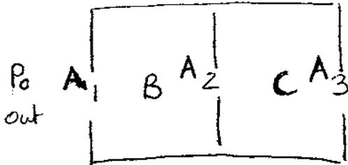
$$\textcircled{1} \quad V_1 = A_1 C_d \sqrt{\frac{2\Delta P_1}{\rho_{out}}}$$
