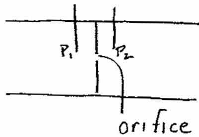
Pressure is measured just upstream and downstream of the small hole in the plate. From a bunch of measurements, the following empirical relationship was derived
