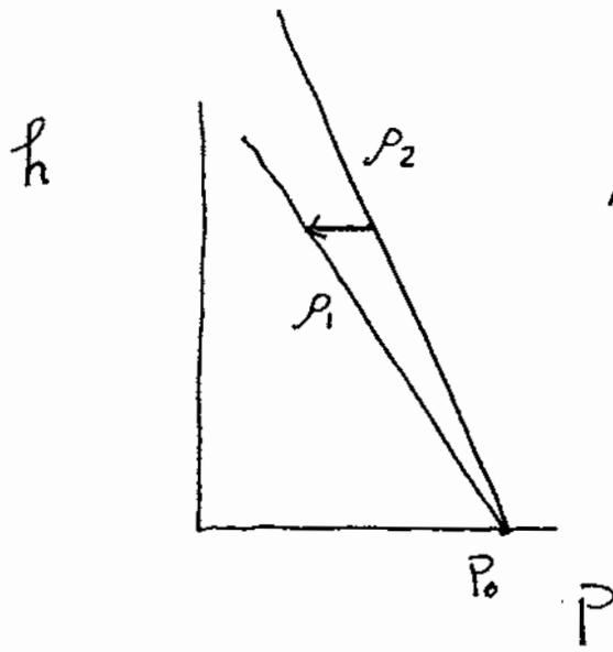
At a given height,  $h$ , air will flow through an opening from the high-pressure side ( $\rho_2$ ) to the low-pressure side ( $\rho_1$ ).
