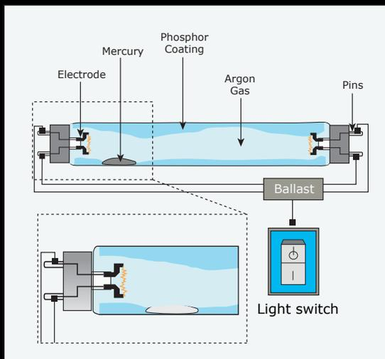
Rapid start and starter switch fluorescent bulbs have two pins that slide against two contact points in an electrical circuit.
