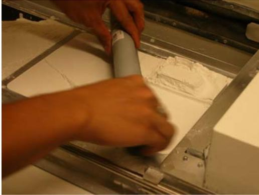
Step 7 – Remove large areas of plaster in the de-powdering box.
