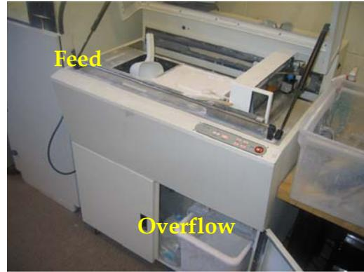
Step 13 – Two scoops of plaster then pack with scoop “make sure the build is all the way up
