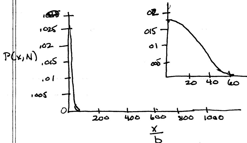
$P(x, N)$  = Probability that in  $N$  steps a freely jointed chain will be  $\frac{x}{b}$  distance from origin
