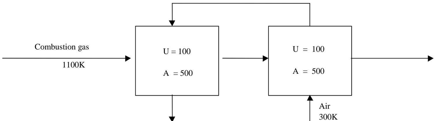
Would scheme (i) or scheme (ii) give the higher air exit temperature? Why? What would the air exit temperature be?
