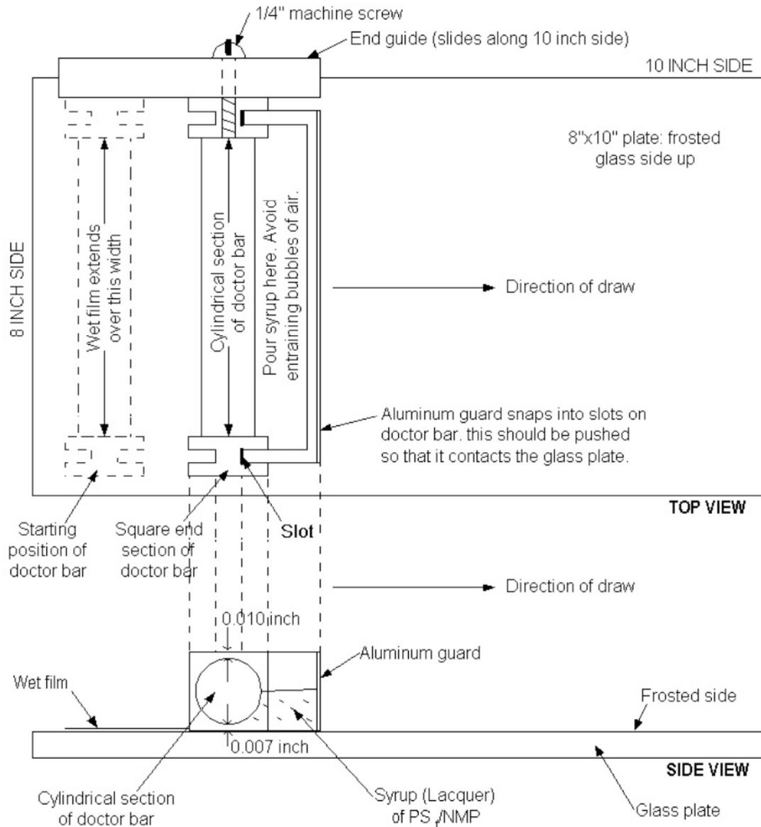
**Figure 5: Membrane casting apparatus**
