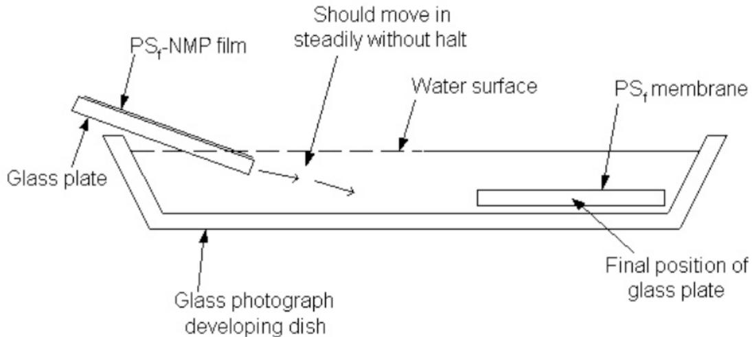
Figure 6: Immersion of the glass plate into the water bath
