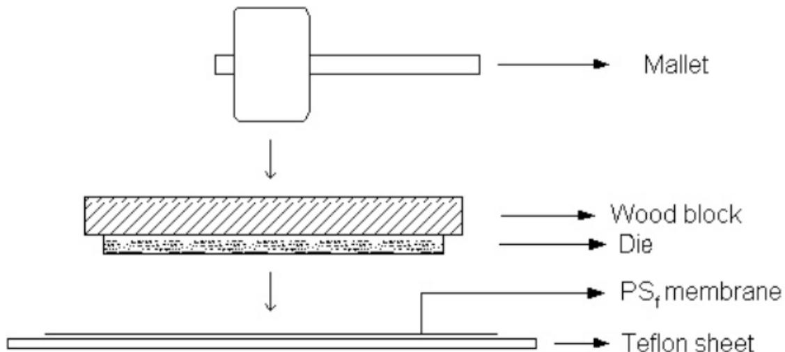
Figure 7: Using the die to cut the membrane
