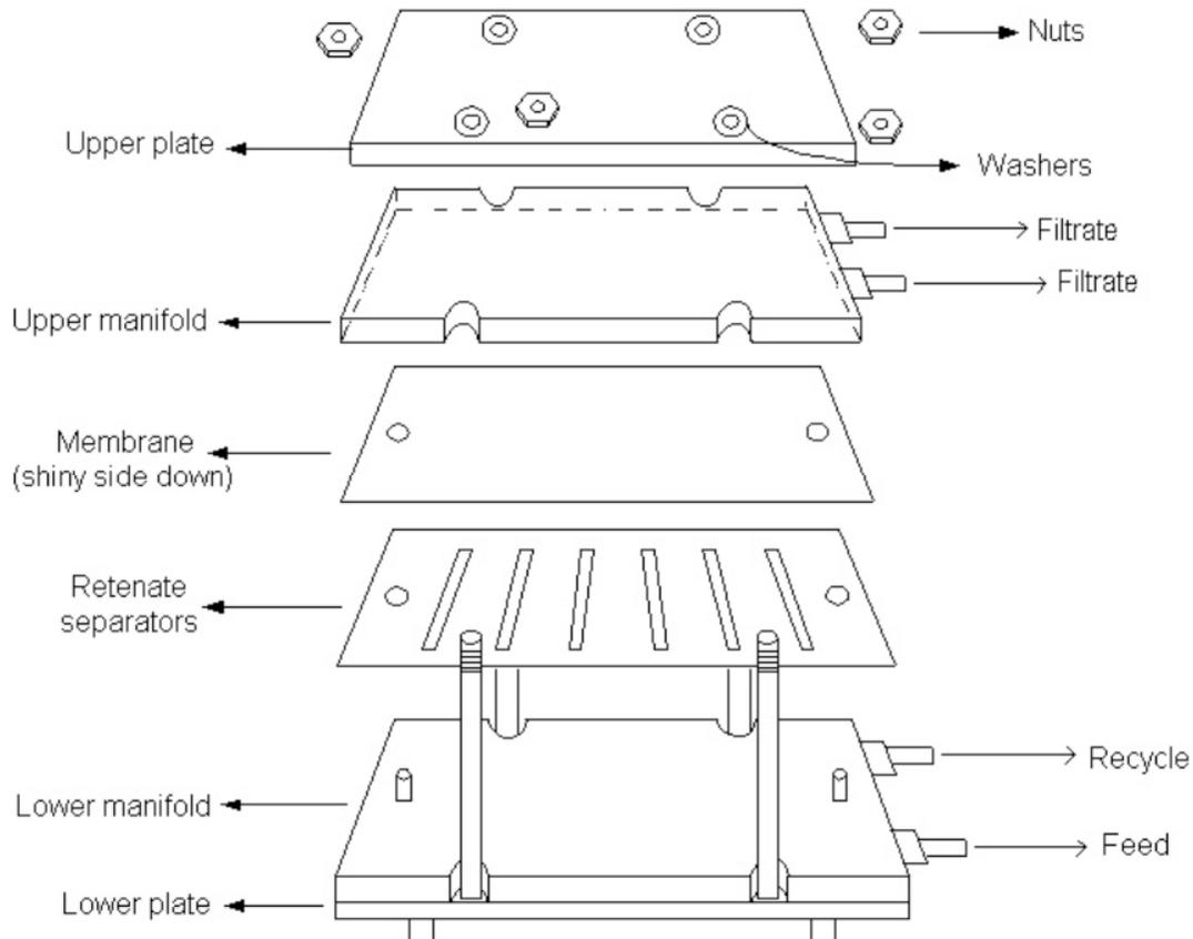
**Figure 8: Installation of the Millipore Corp. Minitan-S module**
