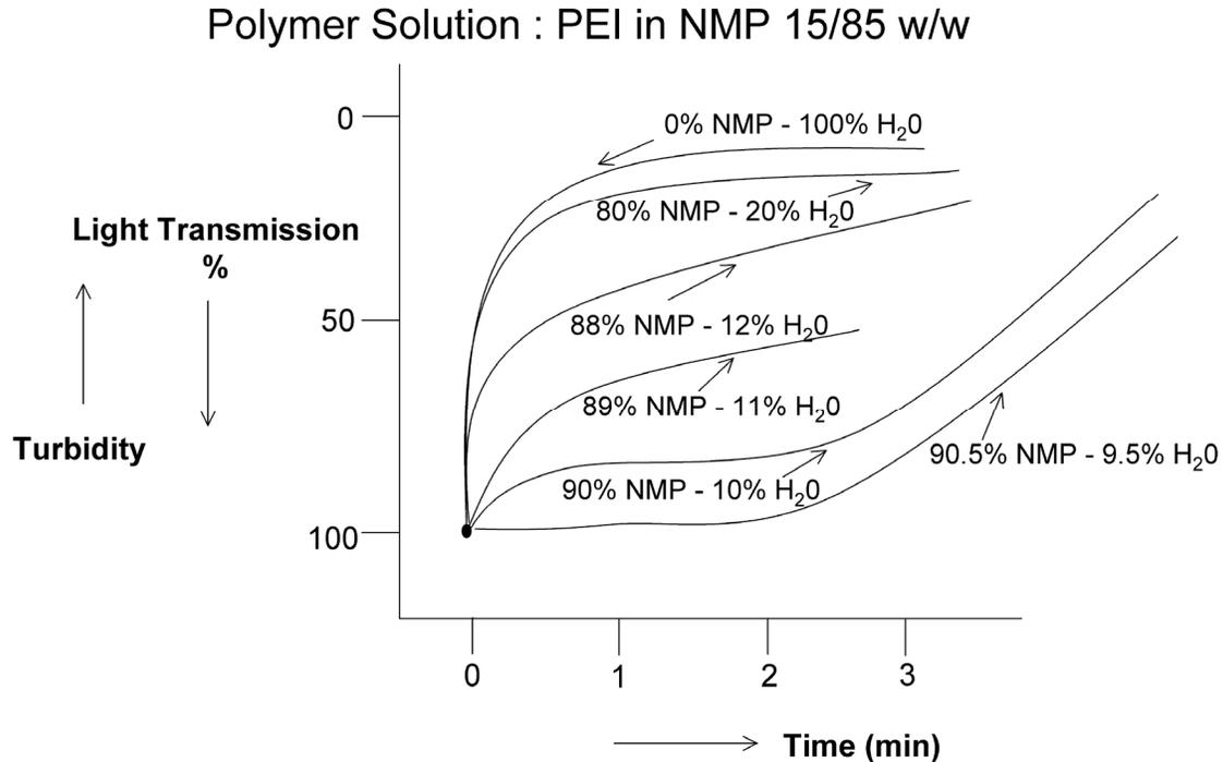
Figure 4: Extent of precipitation of PEI with time as a function of bath concentration
