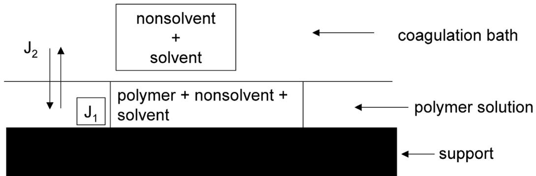
Figure 2. Schematic representation of processes after immersion in a nonsolvent bath;  $J_1$ : nonsolvent flux,  $J_2$  solvent flux
