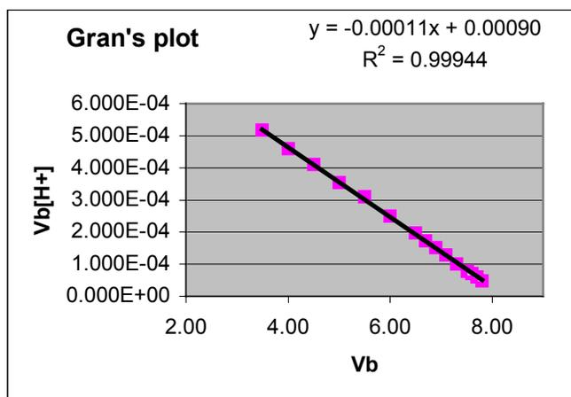
Fig. 5. The linear segment of the titration curve (Gran's plot). The calculated  $K_a$  is  $1.1*10^{-5}$  and  $V_e$  is 8.16 mL of 0.0997 M NaOH (by SD method  $V_e = 8.22$  mL, see above).
