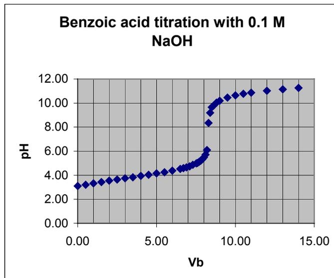
Fig. 2. Typical plot of a potentiometric titration to determine the equivalence point (end point, stoichiometric point) and the  $pK_a$  value. The case of benzoic acid titrated with 0.0997 M NaOH. The y axis is the pH axis, x axis represents the amount in mL of the added base (volume of base,  $V_b$ )
