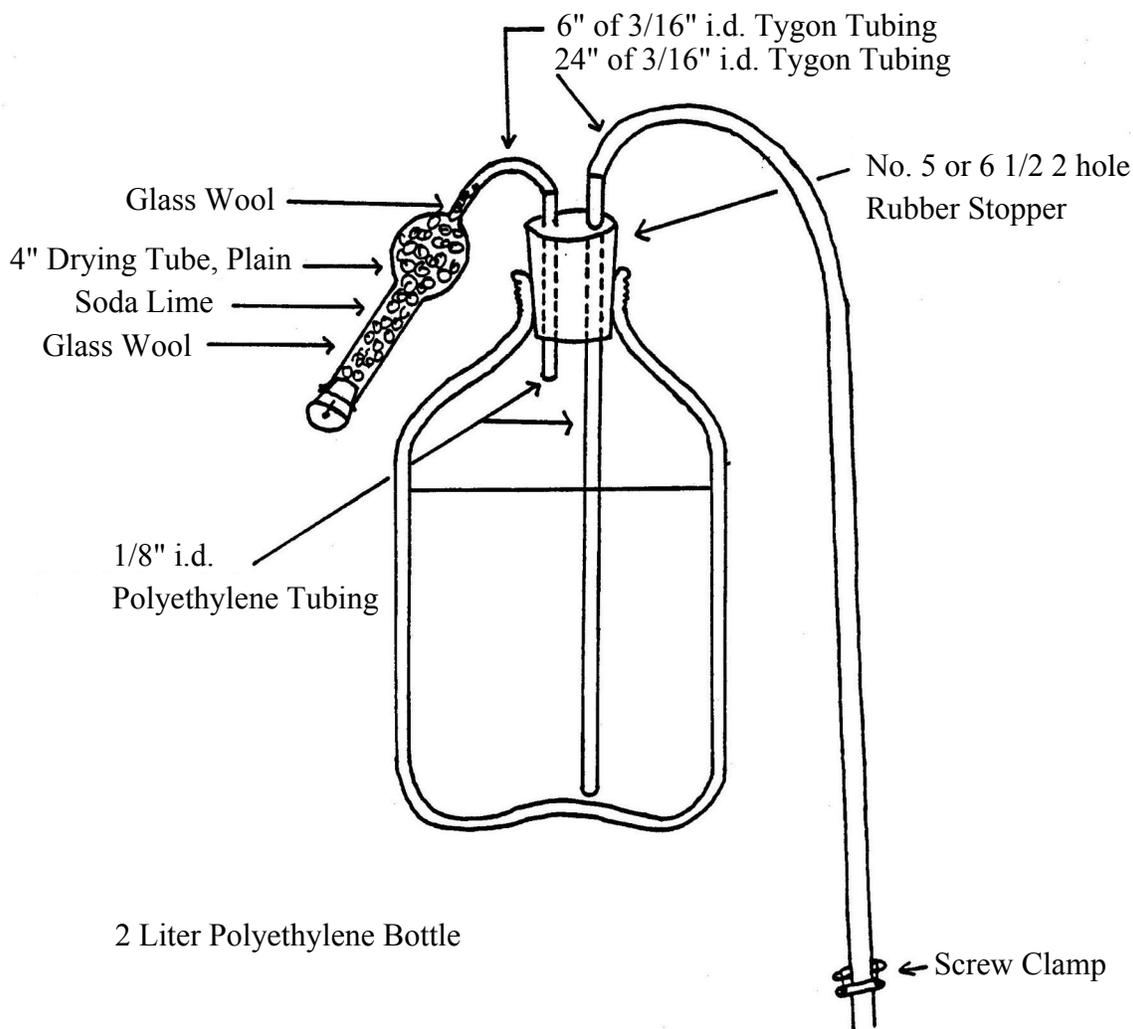
Fig. 1. Siphon storage bottle for standard NaOH
