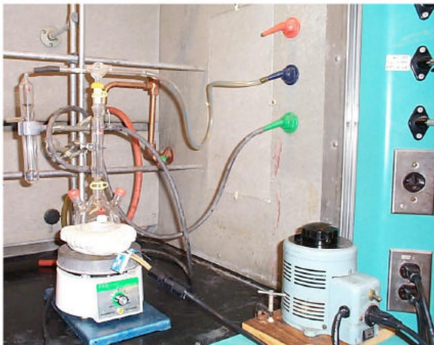
Fig. 2. Apparatus for benzoylation of dibenzyl tartrate.
