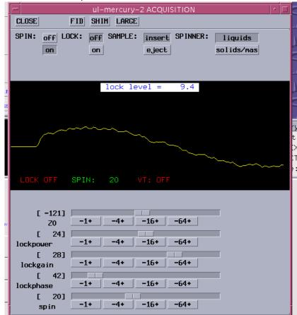
• If the amplitude is too low, increase the **Lock Gain**, and, if necessary the **Lock Power**<sup>2</sup>, until the signal is between 50% and 100%. Continue to adjust **Z0** until one wavelength is seen, and then click the **Lock on** button. The lock step function shown below should appear.
