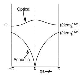
Atoms within each unit cell move out of phase but phases within each cell are identical
