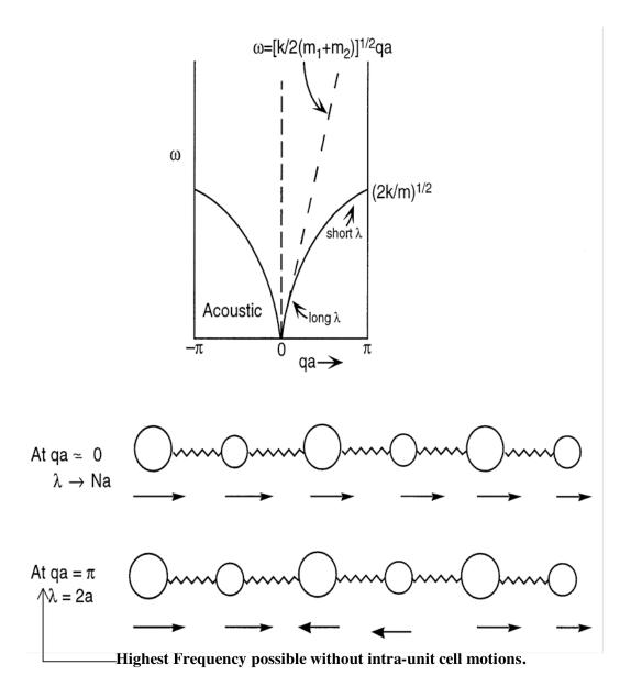
In acoustic modes, both atoms in each unit cell move in phase. At qa = p, both atoms move in phase but phase changes from one unit cell to the next unit cell.
