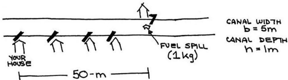
You own a house and dock along a long boat canal. One day your neighbor has a small fuel spill. Due to the boat traffic, the diffusivity in the canal is quite high,  $D = 0.01 \text{ m}^2/\text{s}$ . The current in the canal is negligible, such that the fuel is transported to your house by diffusion only. Assume the fuel mixes rapidly across the width and depth.
