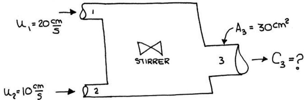
Two pipes, each of  $10 \text{ cm}^2$  cross-section, carry water into a mixing chamber. The upper pipe carries water saturated in oxygen ( $C_1 = 9 \text{ mg/l}$ ), and the lower pipe carries deoxygenated water ( $C_2 = 0 \text{ mg/l}$ ). A stirrer within the chamber rapidly mixes the two streams, such that the concentration in the tank is spatially uniform. Assuming the system is at steady state, what is  $C_3$ ?
