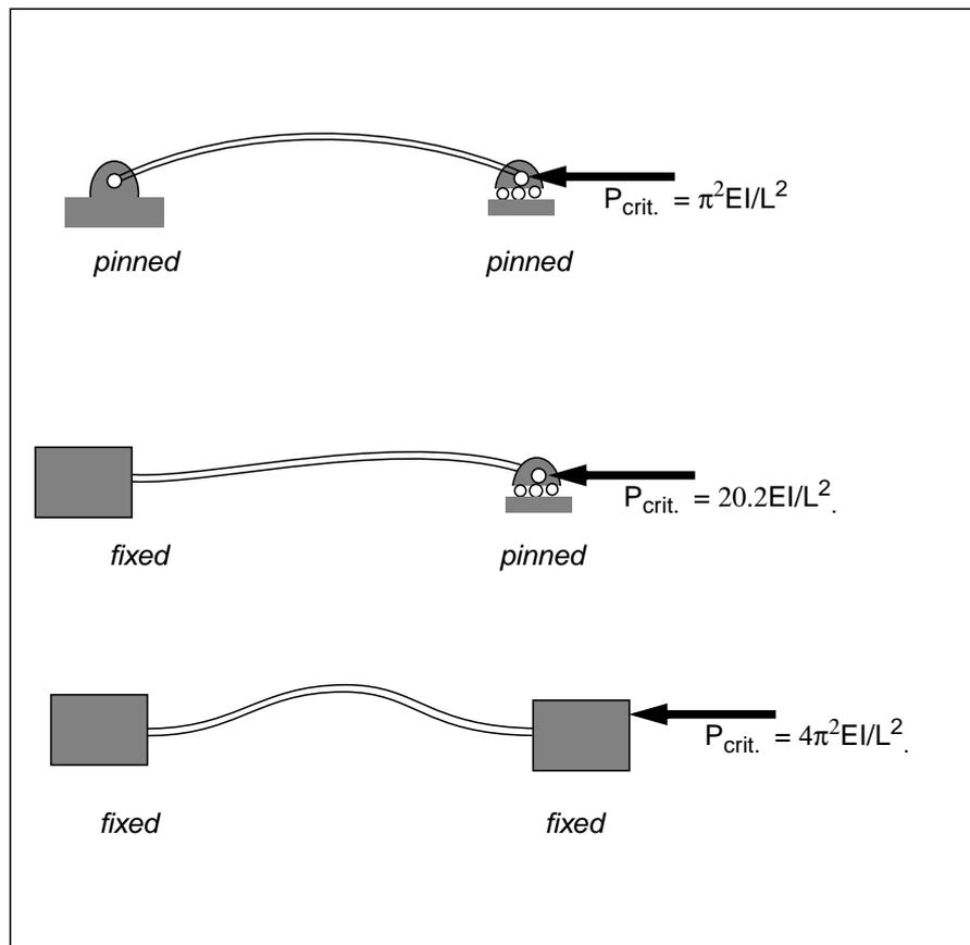
For a circular cross section of radius  $r$   $I = \pi r^4 / 4$ .
