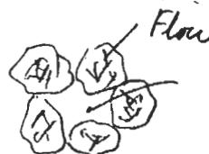
Flow mainly controlled by voids between flocs
