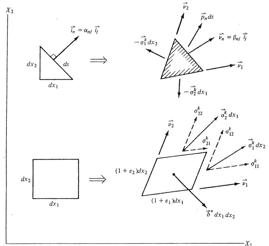
Fig. 10-12. Definition of stress components in Lagrangian representation.
