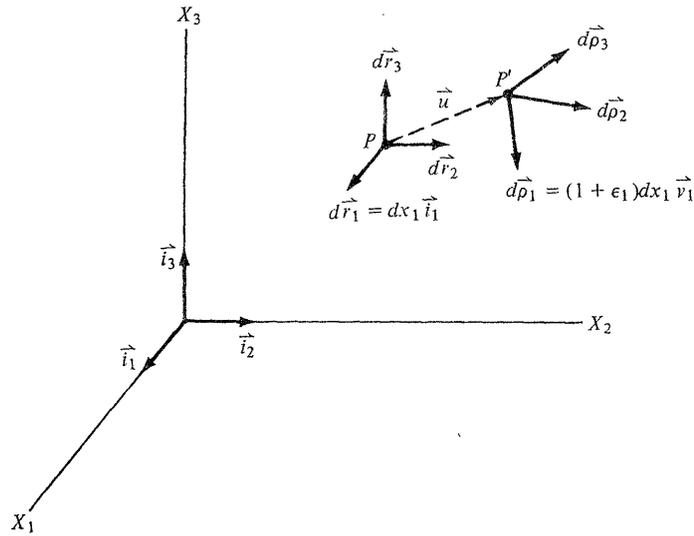
Fig. 10-6. Initial and deformed geometries.
