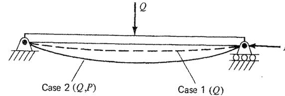
Fig. 10-5. Example of linear and geometrically nonlinear behavior.
