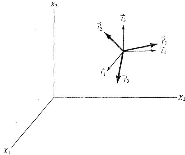
Fig. 10-3. Unit vectors defining transformation of orthogonal directions.
