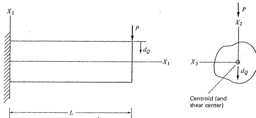
of the member shown in Fig. E12-5. We suppose that transverse shear deformation is negligible, and take the relation between  $k_3$  and  $M_3$  as
