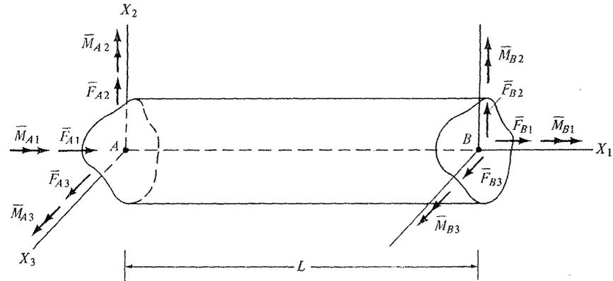
Fig. 12-2. Notation and positive direction for end forces.
