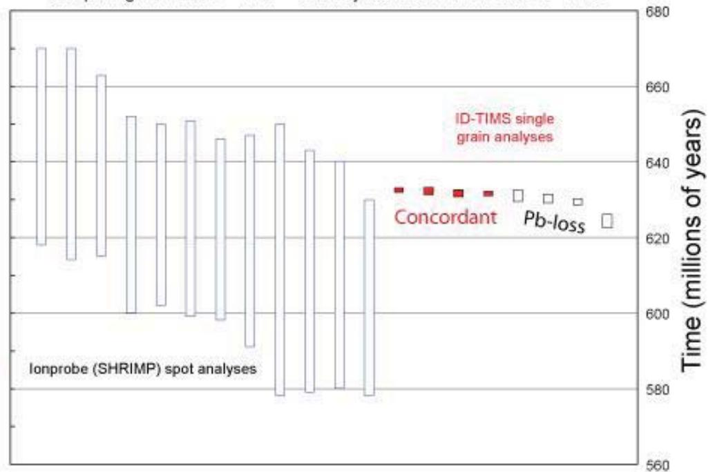
Precise analyses on single grains permits evaluation of scatter in data prior to calculating weighted mean dates from  $n$  analyses.
