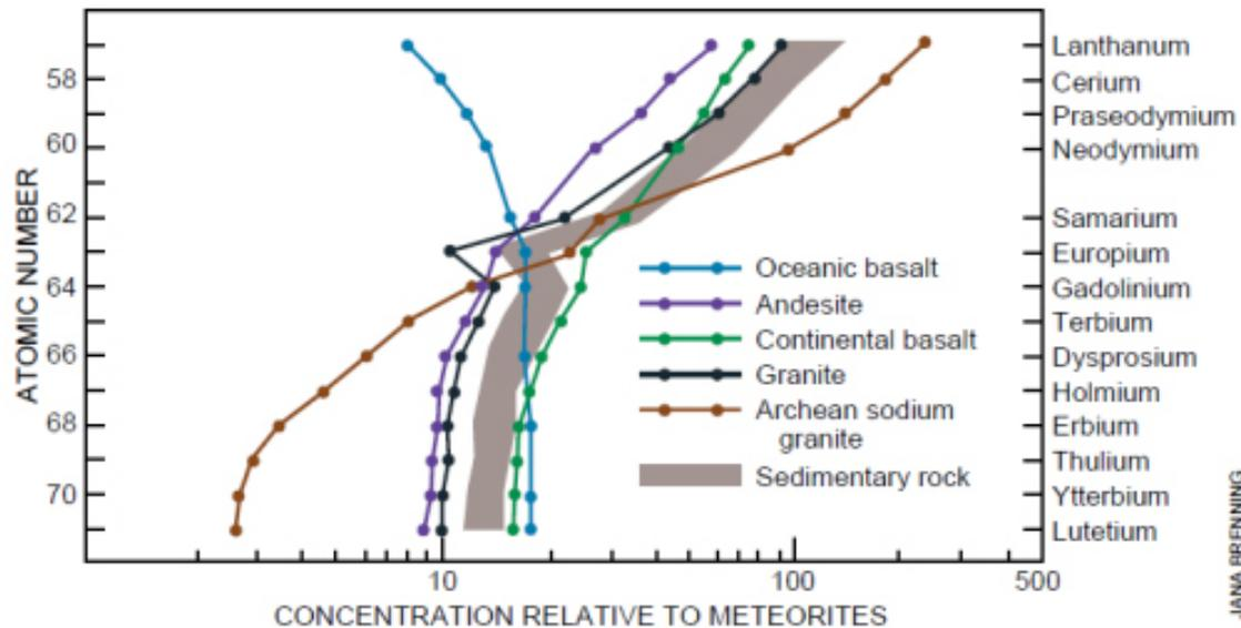
RARE-EARTH ELEMENT abundance patterns provide characteristic chemical markers for the types of rock that have formed the earth's crust. Although igneous rocks (those that solidify from magma) can have highly variable rare-earth element signatures (*dotted lines*), the pattern of sedimentary rocks falls within a narrow range (*gray band*). That uniformity indicates that sedimentary rocks record the average composition of the upper continental crust.
