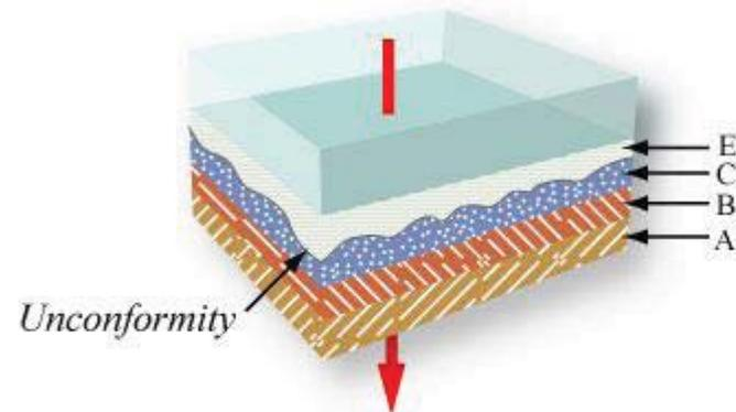
*Subsidence below the sea and sedimentation of E over C; erosion surface of C preserved as an unconformity*
