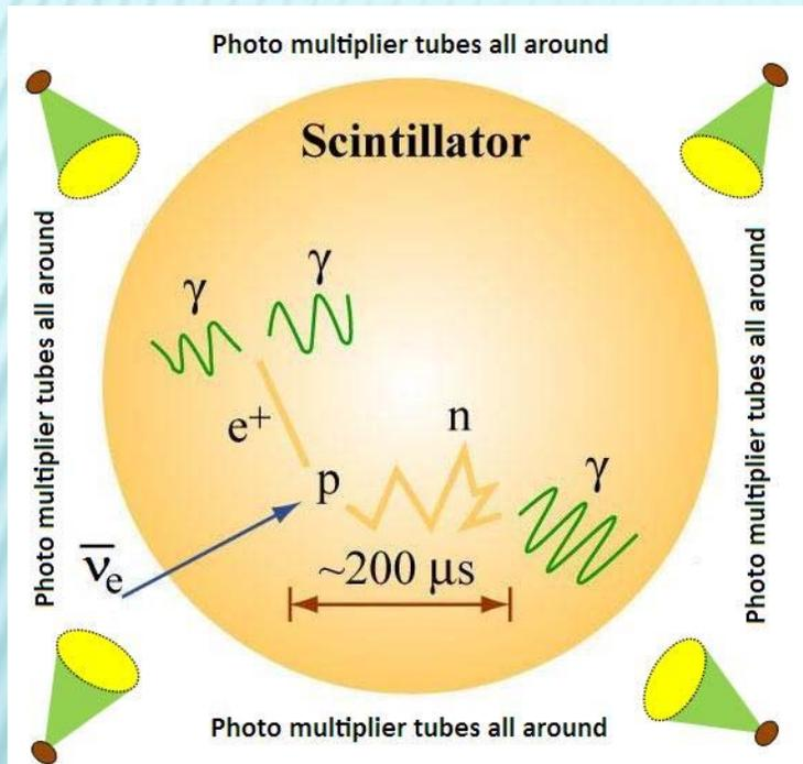
Figure. Pictorial depiction of incident antineutrino detection by inverse beta decay reaction.
