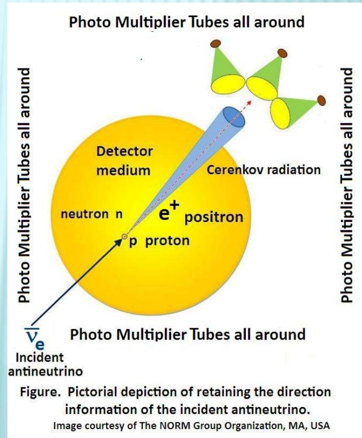
Figure. Pictorial depiction of retaining the direction information of the incident antineutrino.
