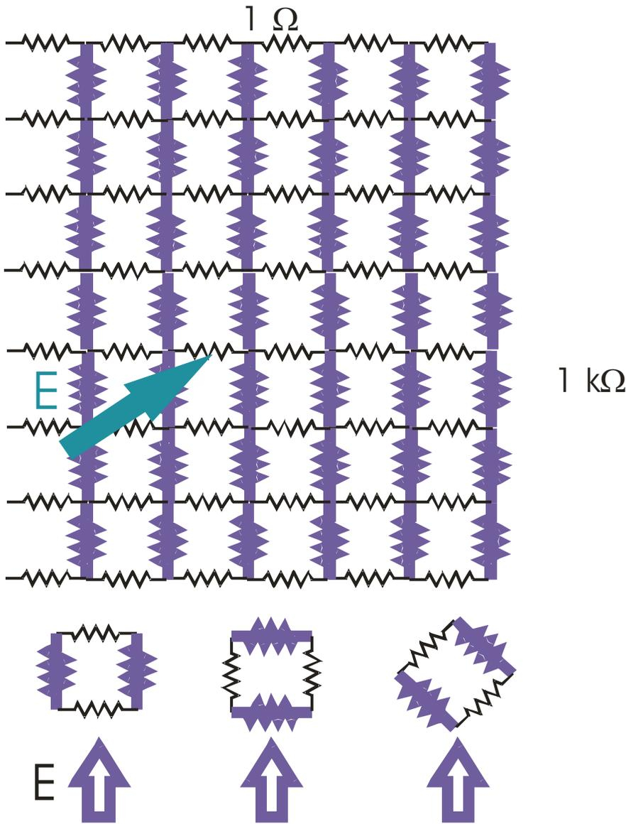
What will be the resistivity in a direction parallel to the 1 ohm resistors? In the direction parallel to the 1 k ohm resistors? In some arbitrary direction in between? What will the indicatrix look like? What does the conductivity tensor look like? What are the principal directions?
