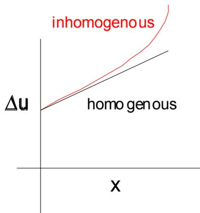
Strain at a point P is the increase in length/original length
