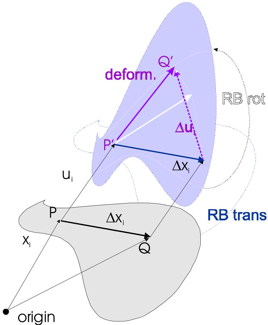
Point  $P$  is carried to  $P'$ ; Point  $Q$  is carried to  $Q'$ . Since we are not interested in the rigid body translation, the deformation can be characterized by the coefficients  $\Delta u_i$ .
