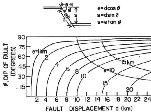
Figure 1: Model for a simple, planar fault
