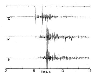
(NB The three components of the seismograms refer to the component of ground motion that is recorded: Z' records the vertical component of ground motion, whereas N' and E' record the North-South and East-West components of ground motion, respectively.
