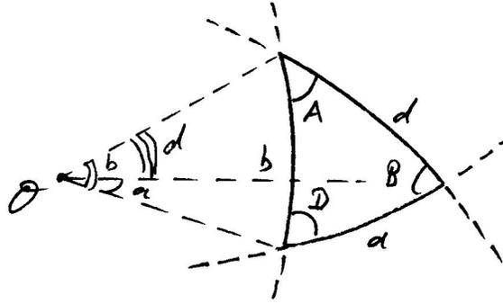
Figure 3.14: Cosine and sine rules on a sphere.
