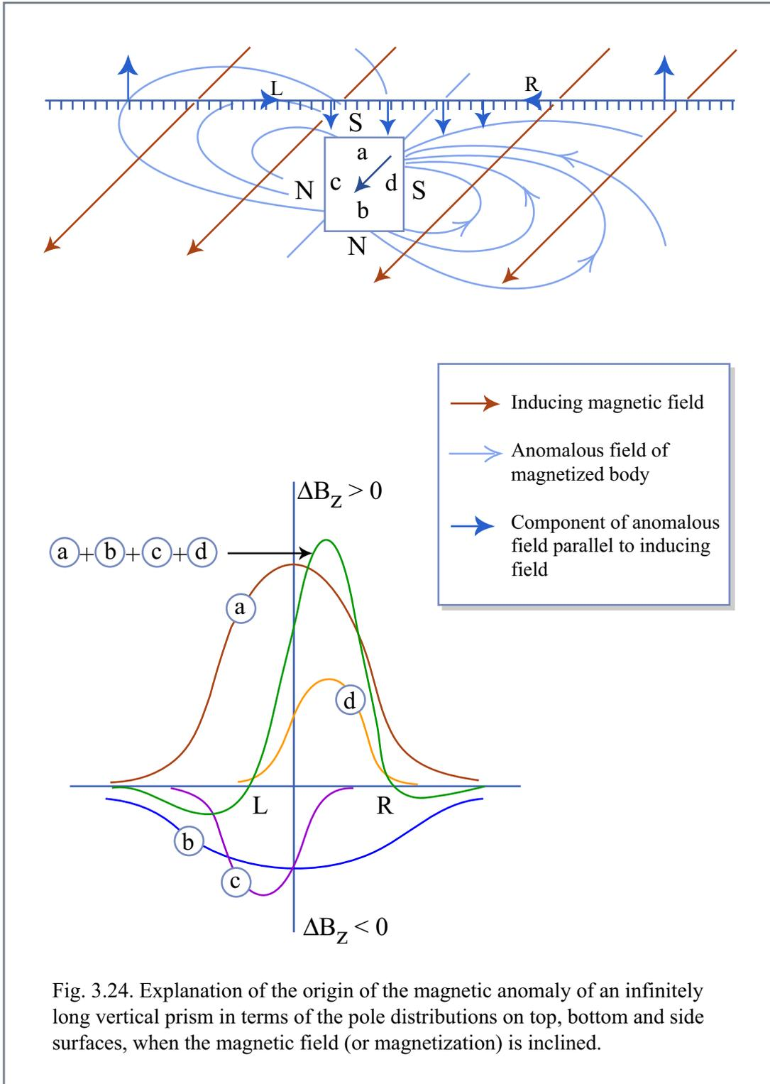
Fig. 3.24. Explanation of the origin of the magnetic anomaly of an infinitely long vertical prism in terms of the pole distributions on top, bottom and side surfaces, when the magnetic field (or magnetization) is inclined.
