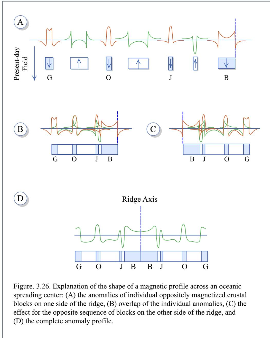
Figure 3.26. Explanation of the shape of a magnetic profile across an oceanic spreading center: (A) the anomalies of individual oppositely magnetized crustal blocks on one side of the ridge, (B) overlap of the individual anomalies, (C) the effect for the opposite sequence of blocks on the other side of the ridge, and (D) the complete anomaly profile.
