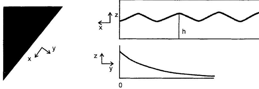
Figure 4.7: Schematic of the trapping of waves at a coast by the planetary rotation. Top figure is in a plane parallel to the coast, which runs along the  $x$ -axis; bottom figure normal to the coast.
