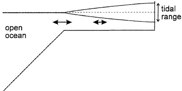
Figure 4.10: Schematic of a quarter-wavelength resonance in a bay.
