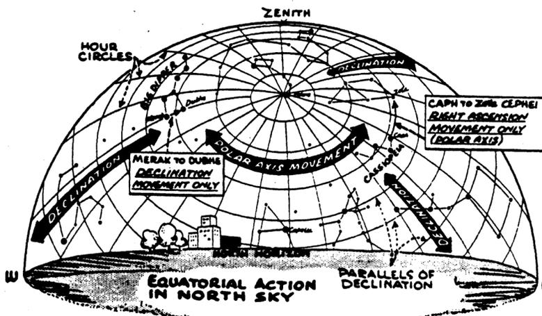
Celestial coordinates take some getting used to. The declination arrows all point north-south — toward and away from Polaris — while east and west are perpendicular to them. An equatorially mounted telescope will move only in these directions. Diagram from *All About Telescopes* by Sam Brown; copyright Edmund Scientific Co.
