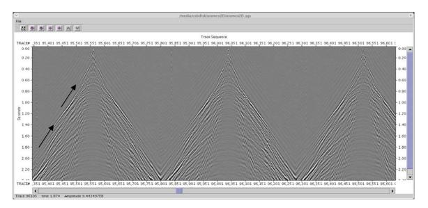
Top arrow points to the direct arrival with limited offsets. Bottom arrow points to delayed refractions from a deeper refractor. The refractions are delayed because of a low-velocity layer above the refractor.
