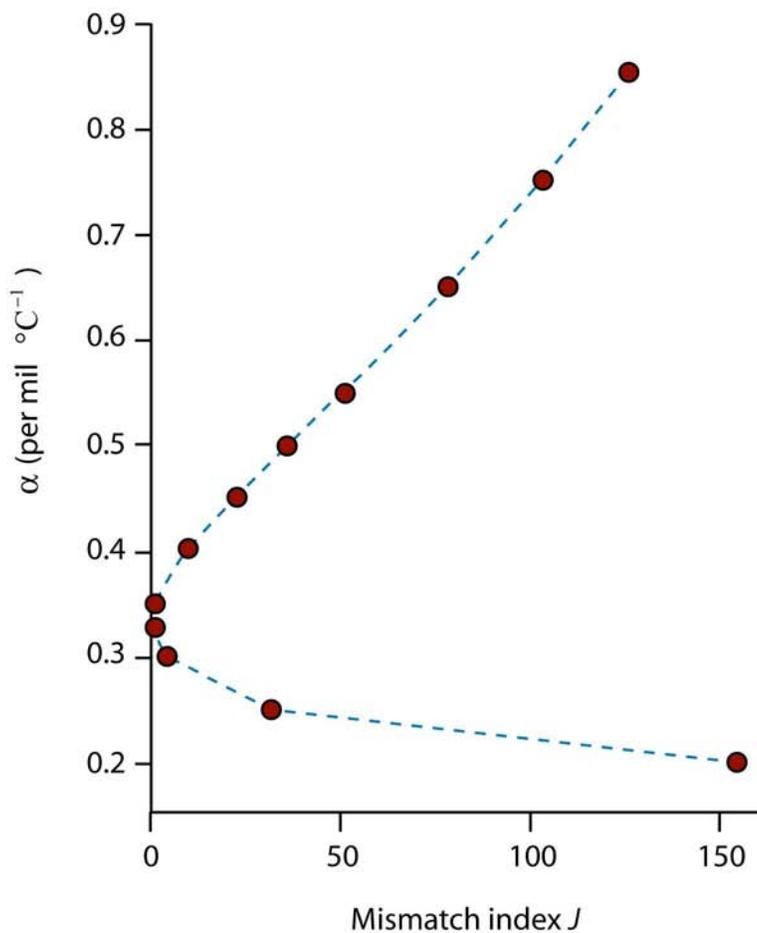
The mismatch  $J$  between modeled and measured borehole temperature profiles, normalized to its minimum value, as a function of  $\alpha$ . The well-defined minimum shows the location of the optimal value for  $\alpha$ ,  $0.327$  per mil  $^{\circ}\text{C}^{-1}$ . To produce this curve, we chose values for  $\alpha$ , then inverted for  $\beta$  and the geothermal flux to optimize the fit.
