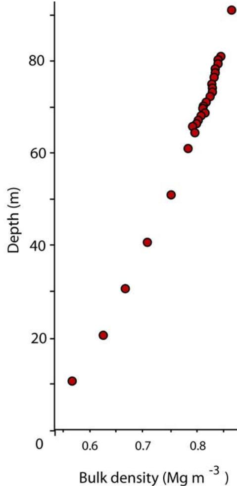
Bulk density and bubble volume versus depth at Siple Station. Each point represents a 1m average.
