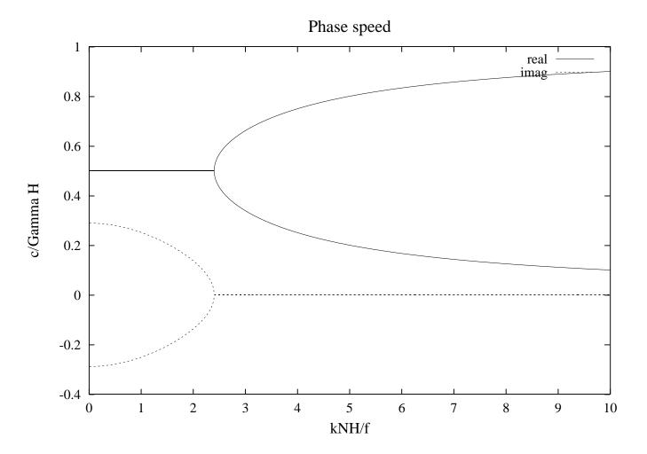
phase speed  $c/\Gamma H$  vs. wavenumber KH
