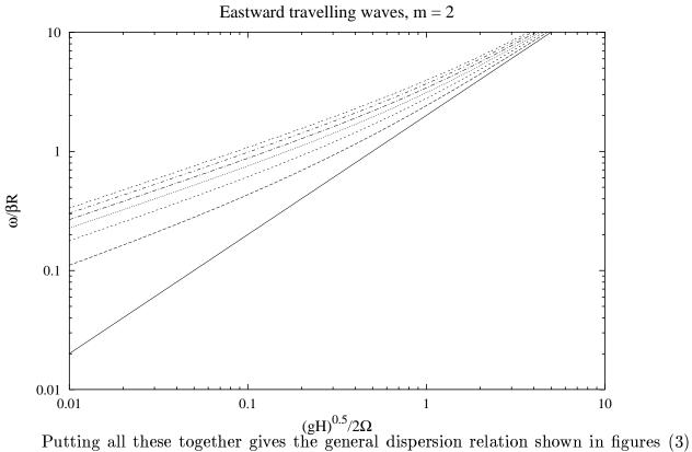
Putting all these together gives the general dispersion relation shown in figures (3) and (4). Essentially, the waves on the equatorial beta plane reproduce the full spherical results fairly well in an analytically simpler regime.
