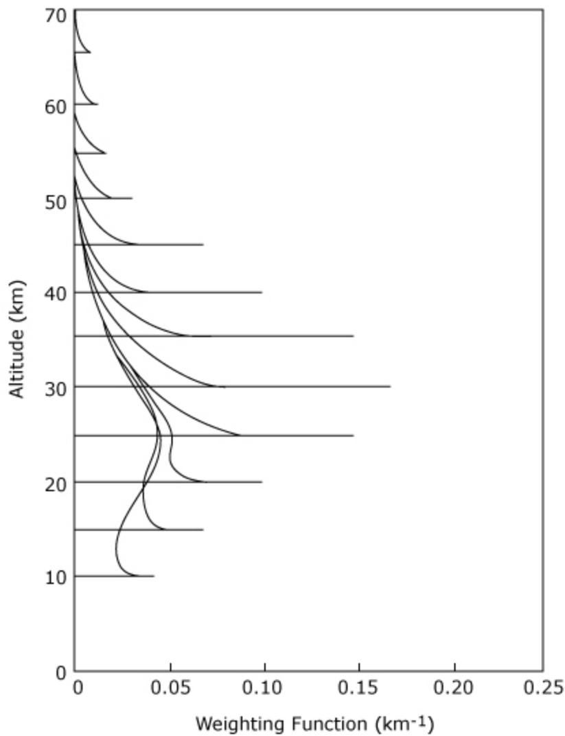
Limb viewing weighting function for the ideal case of an instrument with an infinitesimal vertical field of view for the spectral band 585-705 cm<sup>-1</sup> covering most of the 15 μm band of CO<sub>2</sub>.
