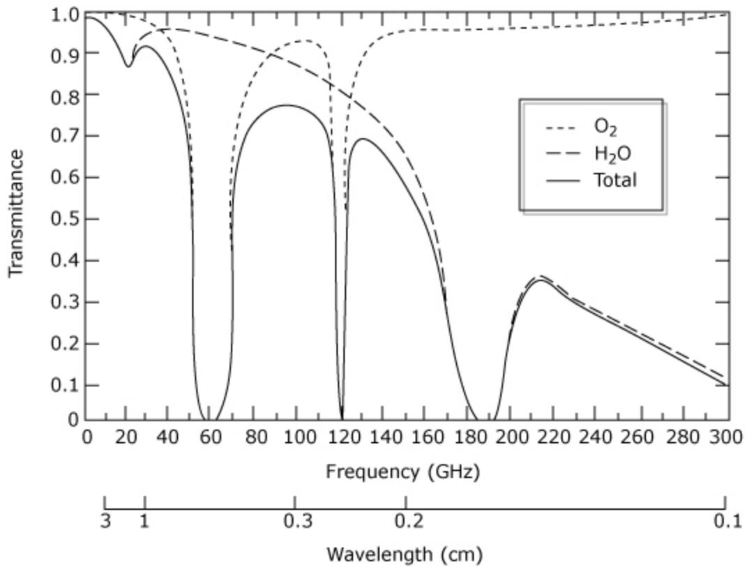
Demonstrative atmospheric transmittances (total, H<sub>2</sub>O, and O<sub>2</sub>) as a function of frequency and wavelength in the microwave region.
