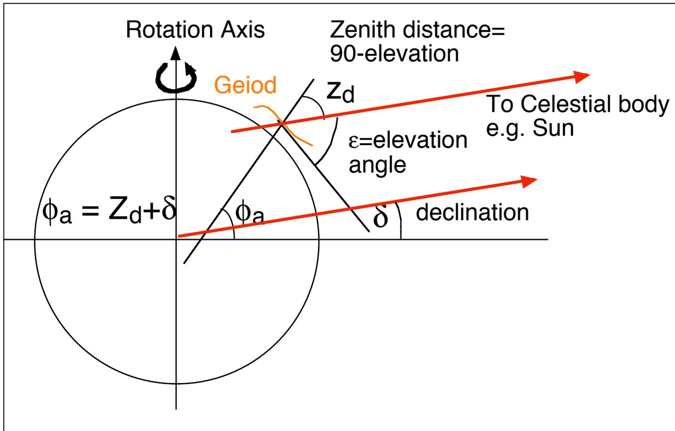
When the sun is at the highest elevation, it is in the plane of the meridian and
