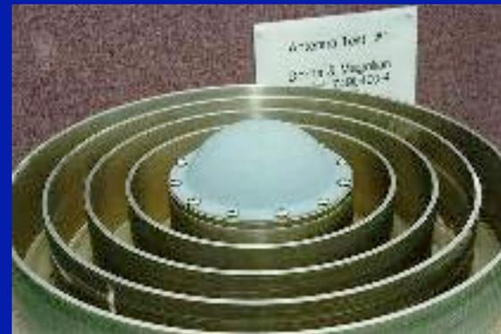
Choke rings and ground plane suppress multipath
