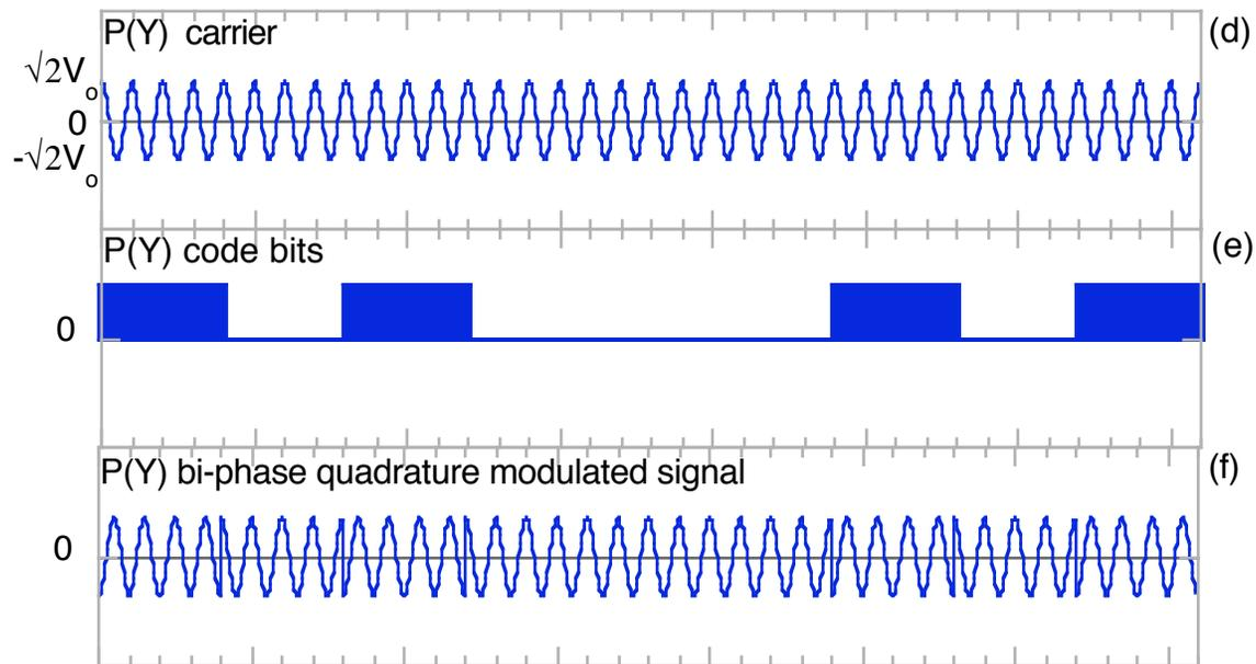
P-code rate should 10 times higher than C/A code
