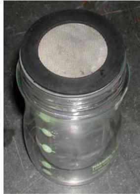
14. Place the spout and screw-on lid on top of the rubber washer and screw the lid tight to seal the elements.
