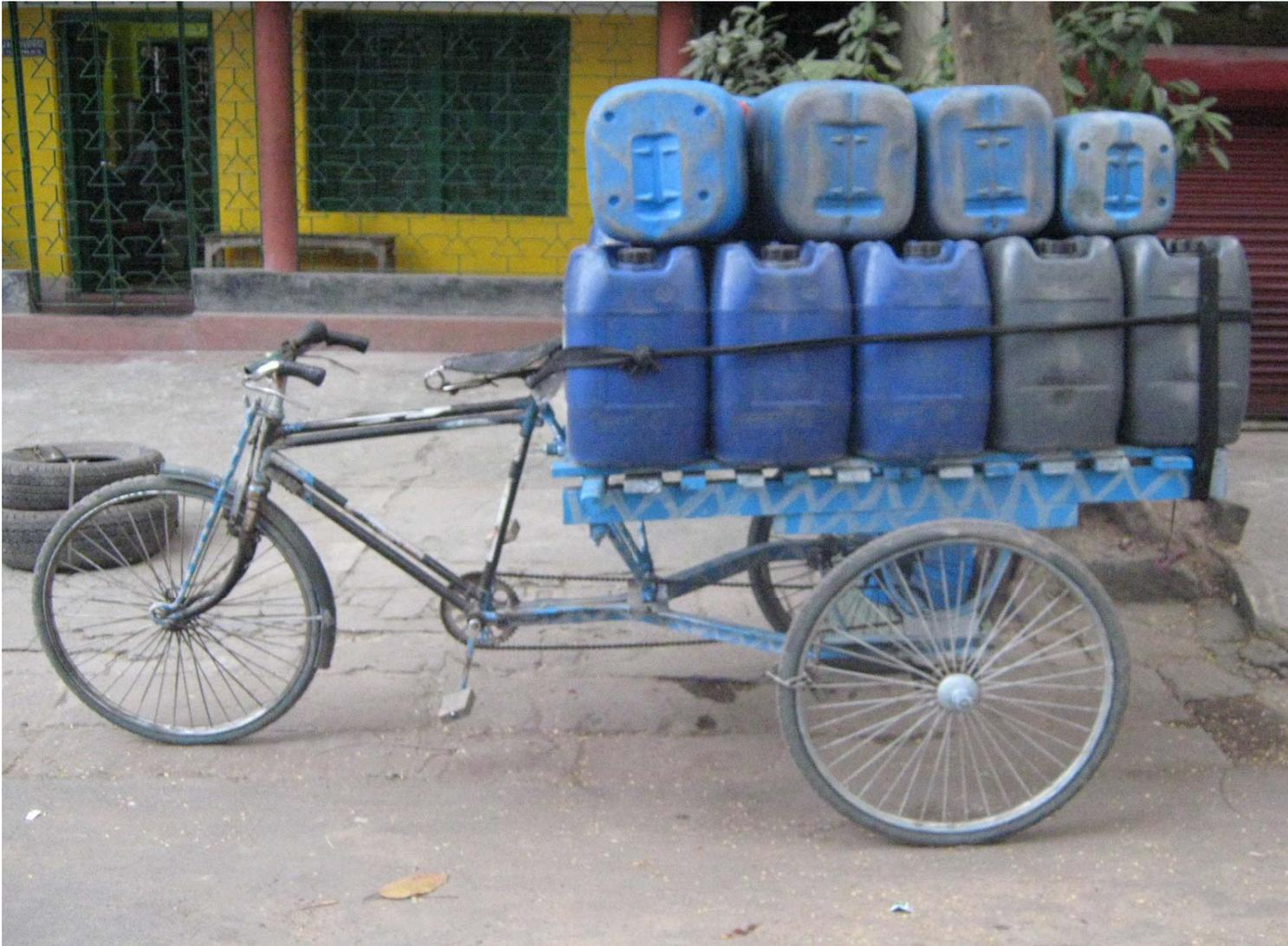
Cycle-van loaded with 880 liters of water. The 23 plastic containers are tied together with the inner tube of wheel tire.
